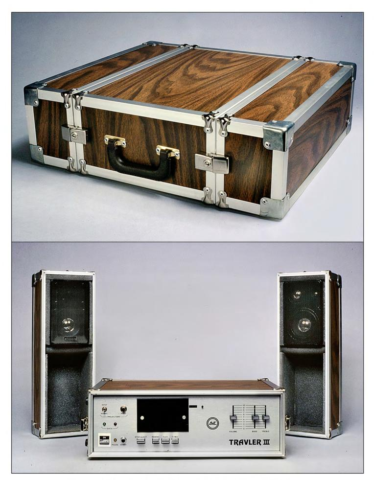
1979 | The Inner World of AVL | Plate N $^\circ$  88 Travler III show in a suitcase | cassette-tape driven playback for up to three projectors.
