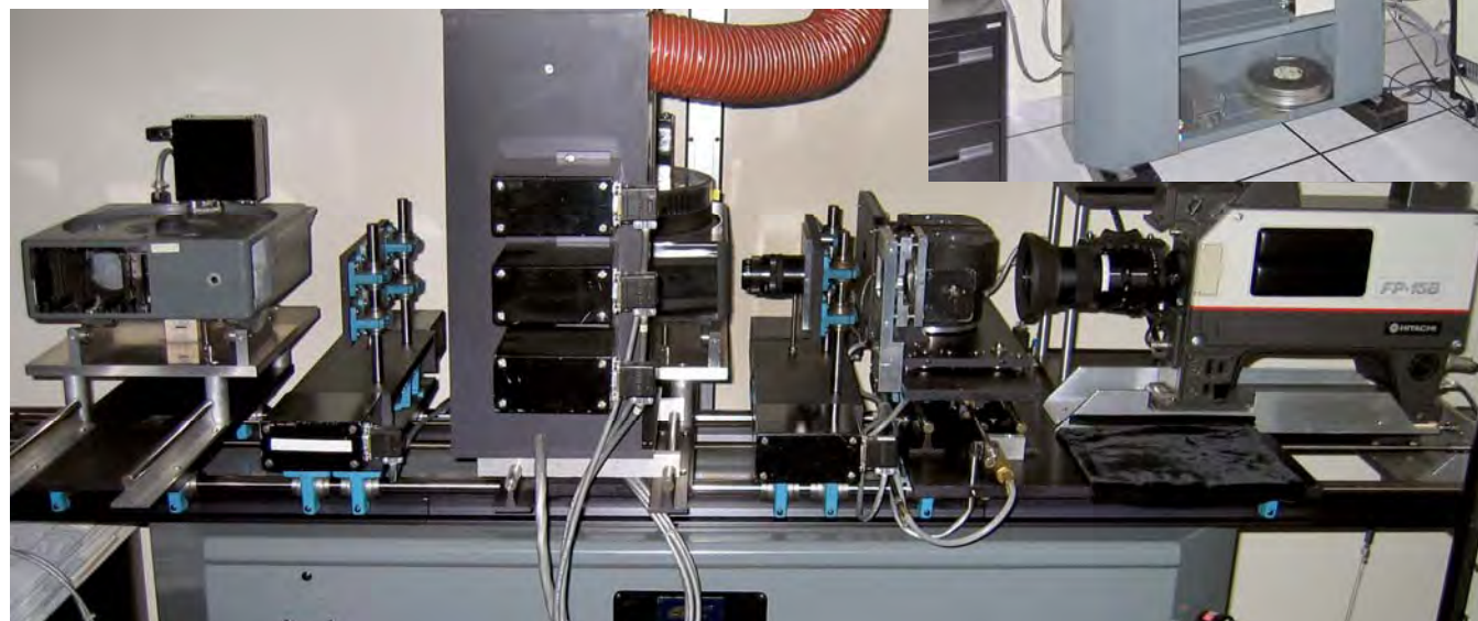
The CAMI slide duplicator operated on the principles of aerial-imaging, discussed earlier [see: 1976 – Buhl Mutiplexer ].
