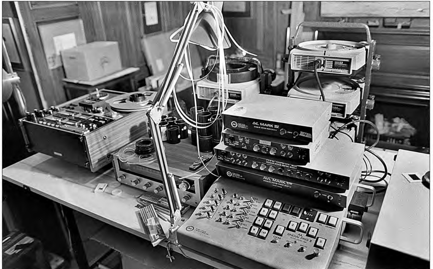
1977 | 23 EAST 73RD STREET STUDIO | PLATE N o 12 Second floor rear | Auxilliary programming | Below: (L) Teac 3340 (R) AVL ShowPro II.
