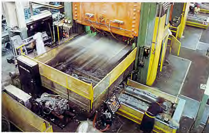
SMC strips for Chevrolet grille opening panels are automatically loaded into 2,000-ton press at General Motors Plant #6, Flint, Michigan.
