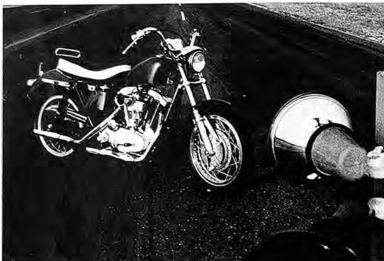
Bike is shown here with a velocity stack; choke and air-filter are used on street.
