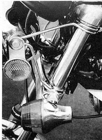
The headlight is insulated from vibrations by rubber grommets. The entire headlight/directional light assembly is mounted on chromed spring steel wires giving the front end a lean, light look—besides saving bulb filaments.
