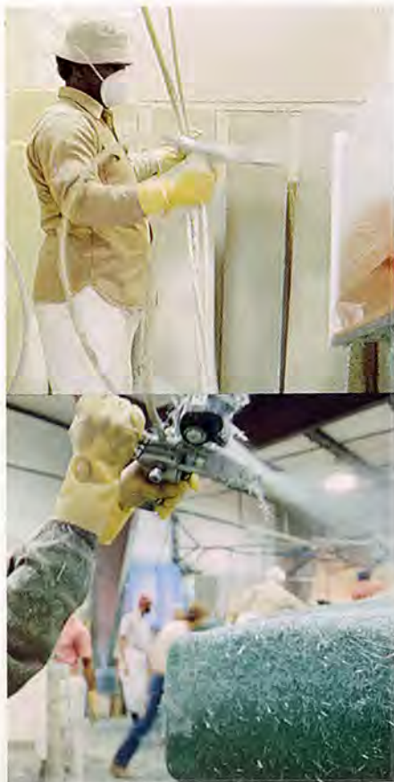
Low capital requirements and the capability for high line speed have made spray-up FRP manufacture popular for large, complex shapes such as plumbing components. Worker first sprays gel coat on mold to give product a smooth, colorful surface. (top) After hardening, coated surface is sprayed to predetermined thickness with resin in fiber glass chopped roving.
