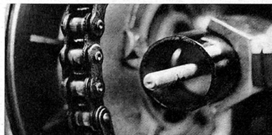
One of the nice touches on the Ducati is the chain adjusters which operate inside the swingarm tubes, making for precise and rigid adjustments.
